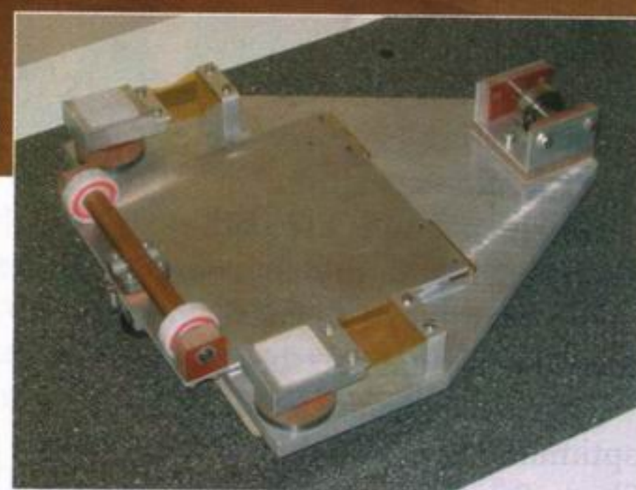
This view shows the underside of the test sled. The two white squares are test pads of perfluoroalkoxy fluorocarbon, or PFA.
